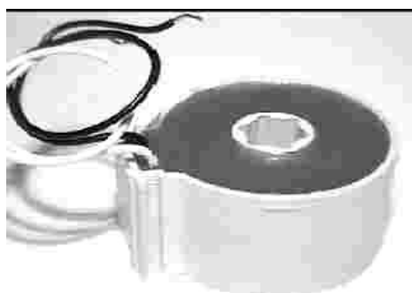
Current Transformer : Custom 2000 Turn Winding on Silicon Iron core and potted in Plastic Case with centre hole for current carrying conductor
