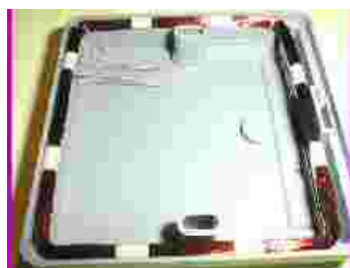
Air Core Coil mounted in Proximity Sensor
