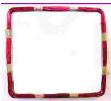
Fig A Air Core Coil for Proximity Sensor
