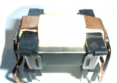
E-Core High power Tape wound Transformer
